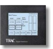
The user panel is a touch-screen LCD with large text and graphic keys. All important information is displayed on the Home screen. Low profile and small size (4" x 4.75") allow for easy mounting.
